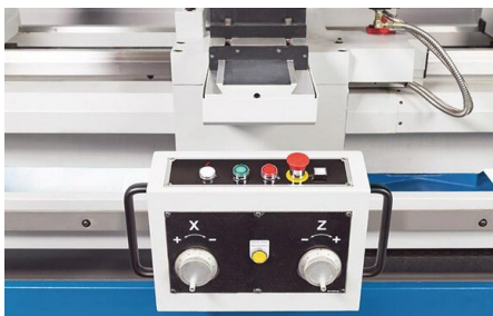
Compact control unit with electronic hand-wheels
